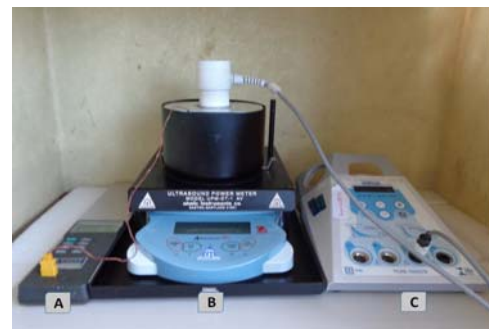
Figure 3: Experimental setup. (A) Digital thermometer, (B) Radiation Force Balance, (C) Therapeutic ultrasound equipment.
