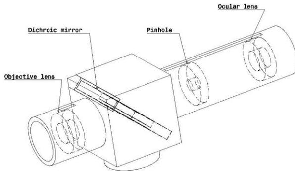
**Figure 2:** optical subsystem that works as a compound microscope with a dichroic mirror.
