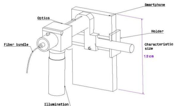
**Figure 1:** View of the complete system high resolution portable microendoscope assembly.
