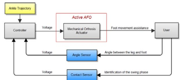
Figure 3: Block diagram of the control system.
