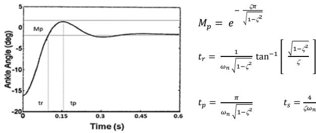
Figure 4: Human ankle trajectory for slow gait speed (0.55m/s).
