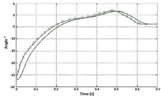
Figure 6: Trajectory tracking of the control with integral action on nonlinear model.
