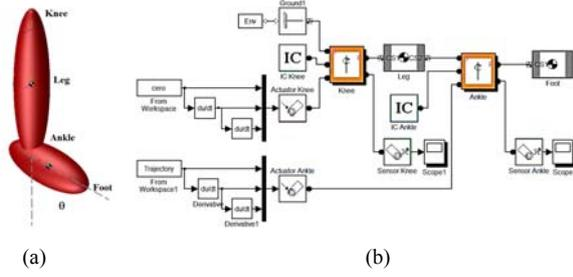
Figure 1: Simmechanics model (a) leg, foot and the ankle joint. (b) block diagram.
