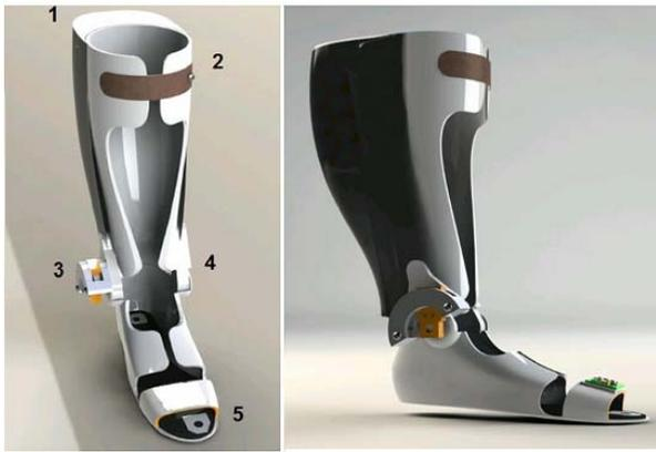
Figure 8: Portable active AFO proposed 1. Power supply and electric circuit; 2. Shank segment ( it can be adjusted to different diameters); 3. Powered joint; 4. Potentiometer, 5. Foot segment and sensor sole.
