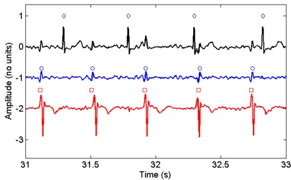
Figure 3: Segment of exemplary NI-FECG extraction using TS (blue) and ICA (red) for maternal SNR = 6dB. Diamonds represent maternal QRS locations, circle and squares represent detected FQRS complex using TS and ICA, respectively.
